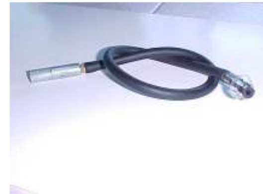
Check valve bleeder. (Photo by Mike Jacobsen.)
