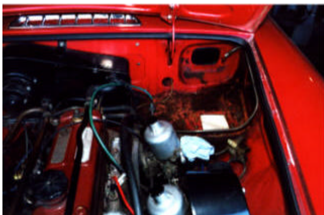
The above photo shows where the brake master cylinder and clutch master cylinder are located in the engine compartment. Soon to be rebuilt! (Photo by Ray Watson.)
